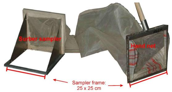
Figure 33: Surber sampler and hand-net
