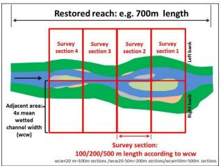
Figure 1: Survey sections - degraded reach
