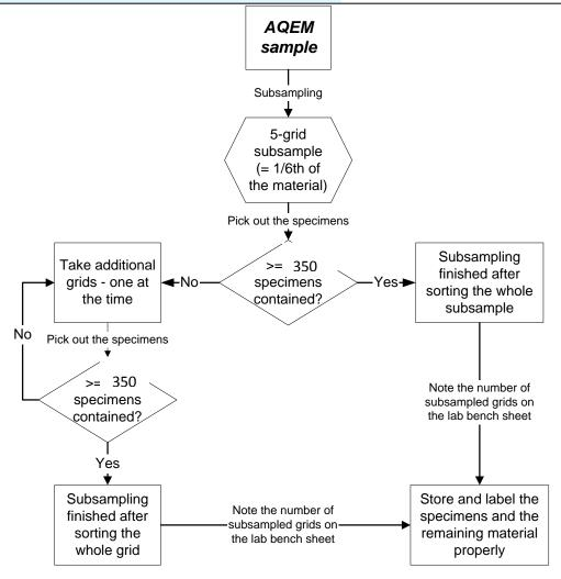
Figure 40: Flowchart of the subsampling procedure. The example is based on the original subsampler after (Caton 1991) with 30 grids, each  $6 \times 6$  cm. A minimum amount of 1/6th of the material has to be subsampled, containing a minimum number of 350 specimens
