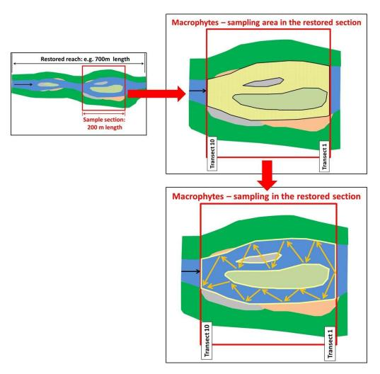
Figure 42: Sampling of maccrophytes in the restored section (sample area is marked in yellow; orange arrows show the way of wading)
