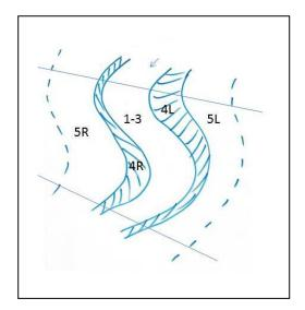
Figure 12: Scheme of spatial relation of - Figure 13: Scheme of spatial relation of the 5 main parameters - braided section 5 main parameter - meandering section 1-3: Channel Geometry and Flow Characteristics / Riverbed / Water - land transition zone; 4: bank and riparian structures (L/R: left/right bank); 5: vegetation of the adjacent area (L/R: left/right riverside)
