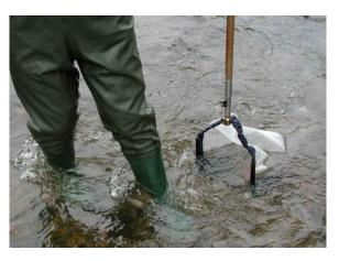
Figure 35: Using a hand-net for jabbing Figure 36: Kick-sampling. and sweeping.
